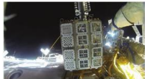
EXPOSE-R2 on the International Space Station with experiment BIOMEX. (Courtesy of ESA).
